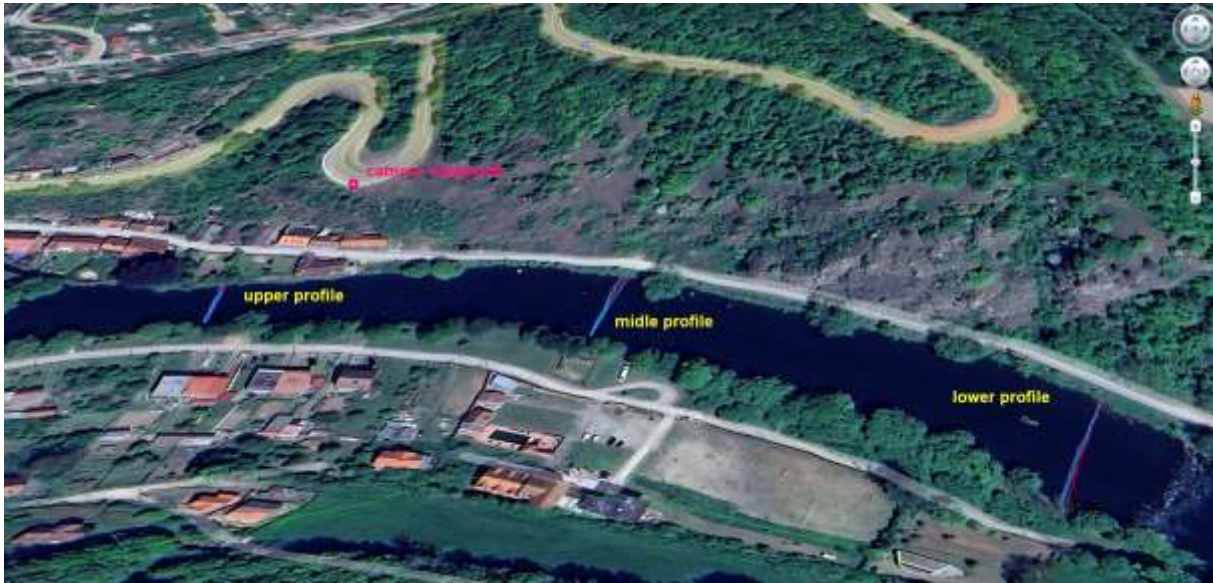
Fig. 13 Aerial view of LSPIV measurements.
