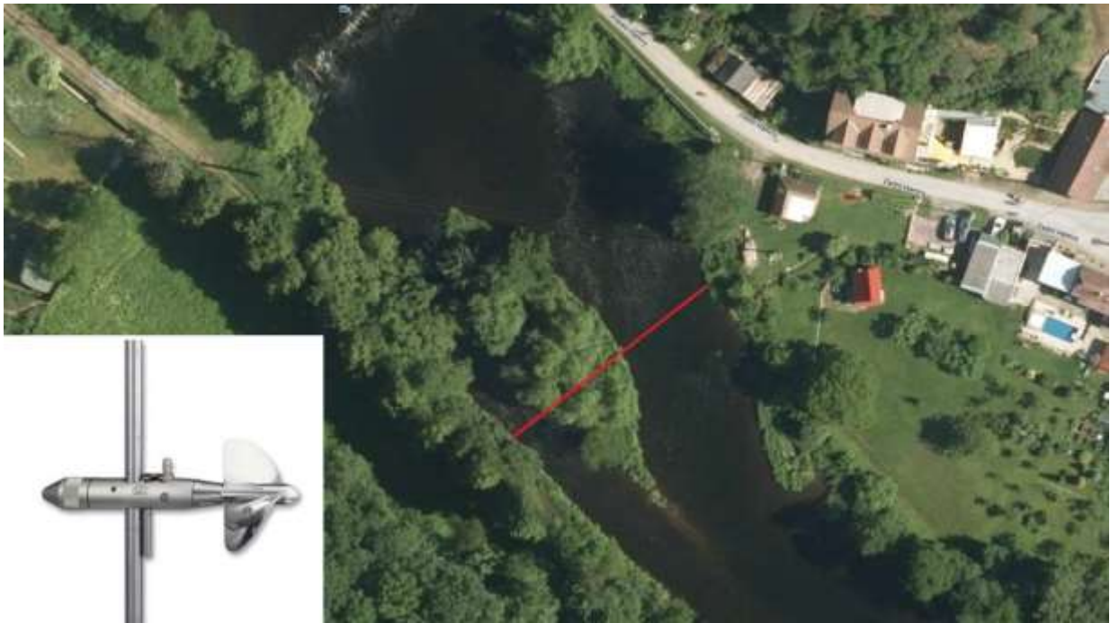
Fig. 8 Ott C31 propeller and location of the measurement
